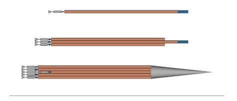
Figure 1. Small Launch Vehicle 931 showing top stage, top two stages, and launch configuration.
