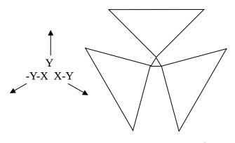
Figure 2. Solar Sail Spacecraft Vehicle Axis Definition.
