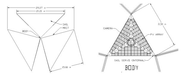
Figure 5 Solar Sail Vehicle dimensions
